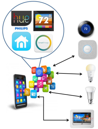
Figure 1: Heterogeneity in today's smart-home IoT systems. Each appliance requires its own app as shown here that requires an appliance-specific user interface for control
