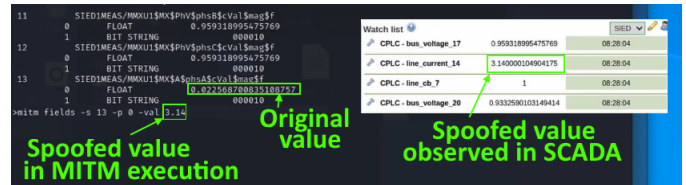
Fig. 6. MITM Attack on a Power Grid Measurement
