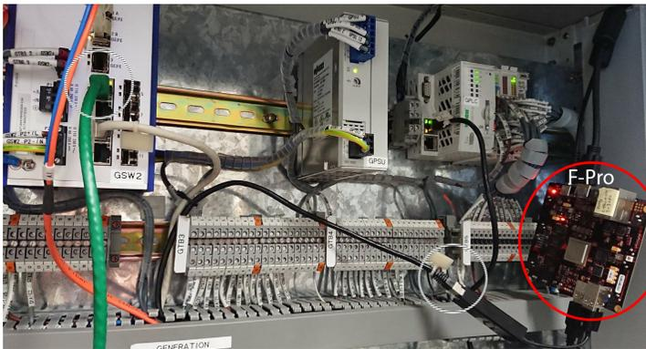
**Figure 4.2:** F-pro Device Deployed in Front of a PLC in the Smart Grid Testbed (Esiner *et al.*, 2019)
